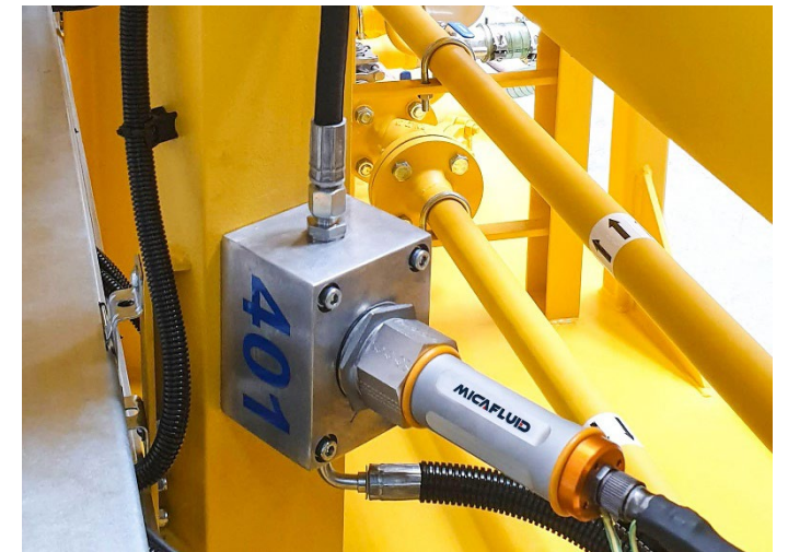
In-line breakdown voltage measurement with MicaSonic™
